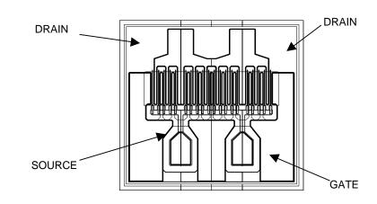
DIE SIZE: 16.5 x 16.1 mils (420 x 410 μm) DIE THICKNESS: 3.0 mils (75 μm typ.) BONDING PADS: 1.9 x 2.4 mils (50 x 60 μm typ.)
